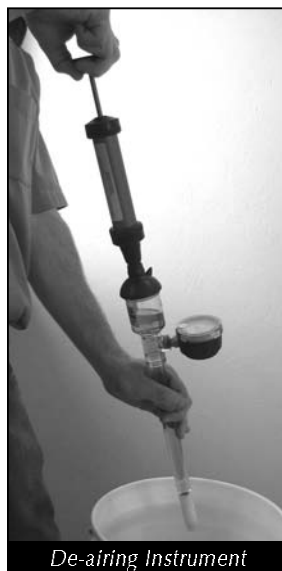
De-airing in the Ground
